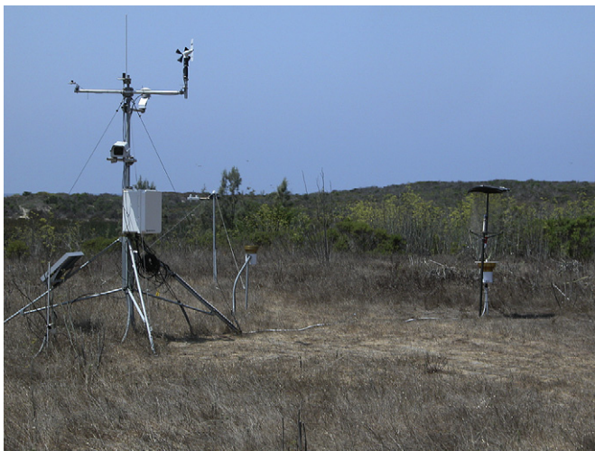
Fig. 1. Coal Oil Point research station. Marine-grade anemometer, pyranometer, cellular antennae, solar panel, camera, temperature/relative humidity sensors, and enclosure with datalogger installed on main tripod. Additional instruments include leaf moisture sensor, rainfall tipping bucket, fog collector, four-channel net radiometer, and soil moisture and temperature probes.
