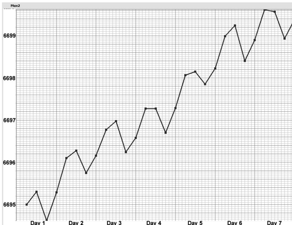
**Figure 4** The trend line shows interesting upward trend with daily fluctuations. These seven days show an increase of the sensor digit readings by five digits
