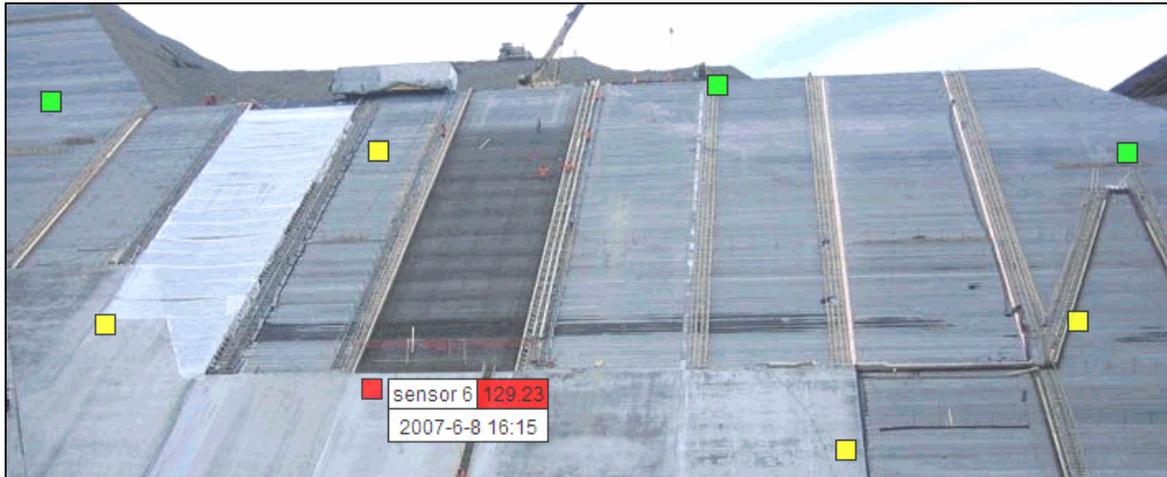
Fig. 5: A web map gives great overview of complex instrumentation. In this figure, a simulated set of sensors show normal status (green), H alarm status (yellow) and HH alarm status (red). The actual readings are visible by clicking on one or more of the sensors (see sensor 6 as example).
